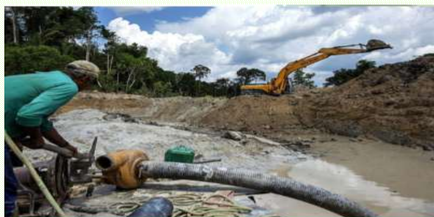
Image 3- Illegal mining activity on indigenous lands in the Das Tropas river tributary of the Tapajós river, use of machines coupled to water hoses called "Tatuzão".
